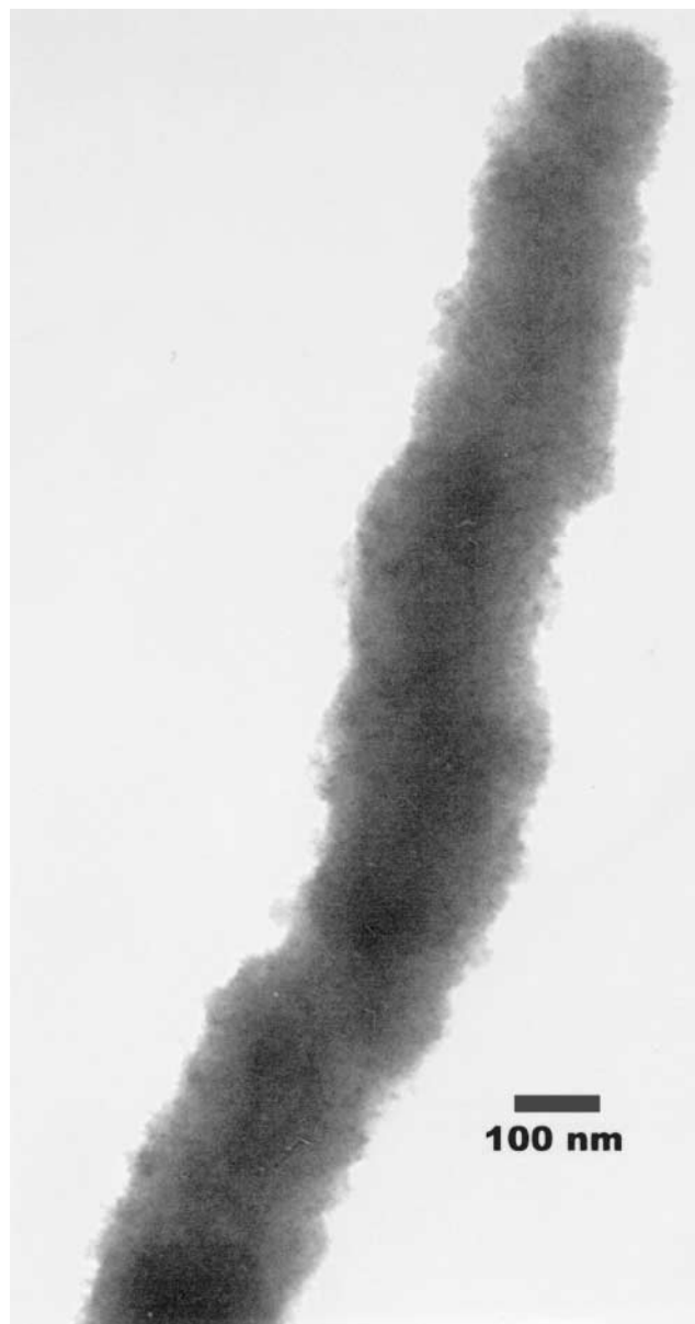
FIG. 3. HRTEM micrograph of an individual acicular iron particle from the collection of iron particles shown in Fig. 2.
